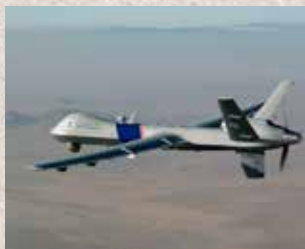
The General Atomics MQ-9 Reaper (formerly named Predator B) is an unmanned aerial vehicle (UAV) capable of remote controlled or autonomous flight operations, developed by General Atomics Aeronautical Systems (GA-ASI) primarily for the United States Air Force.
